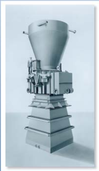
AirPol Blast Furnace Venturi, silicon carbide brick lined with double damper adjustable throat for 500,000 ACFM.
