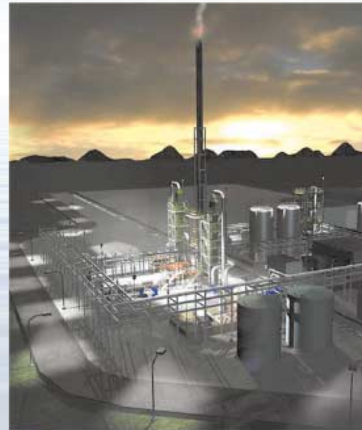
AirPol air pollution control system consisting of two quench-absorber trains for a hazardous waste incinerator plant.
